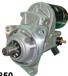
SN-0850 4.5kw, CW, 11T OEM:028000-850
